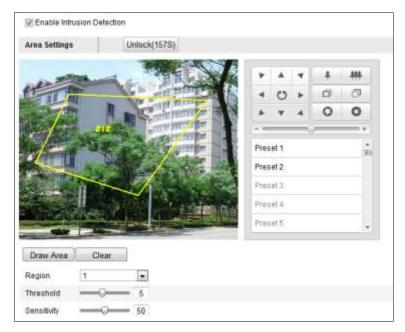
Figure 6-52 Configuring Intrusion Area
