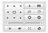
Figure 4-3 PTZ Control Panel
