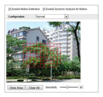
Figure 6-41 Motion Detection Settings-Normal
