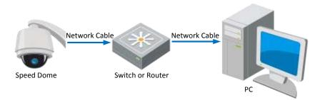
Figure 2-2 Connecting via a Switch or a Router
