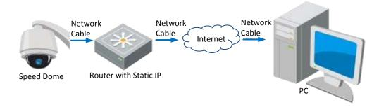
Figure 2-4 Accessing the Speed Dome through Router with Static IP
