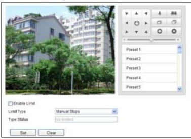
Figure 5-3 Configure the PTZ Limit
