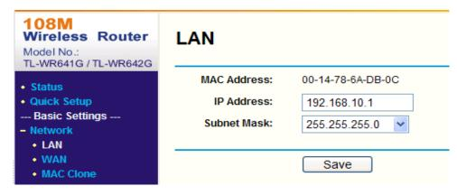
Figure A.2.2 Set the LAN parameters
