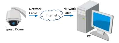
Figure 2-5 Accessing the Speed Dome with Static IP Directly
