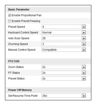
Figure 5-2 Basic PTZ Configuration Interface
