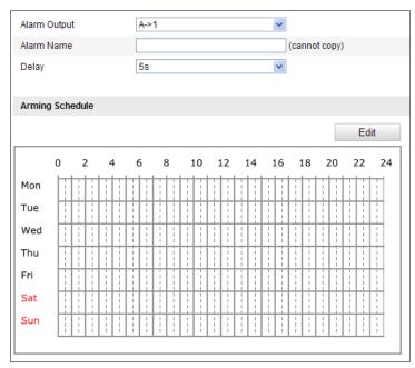
Figure 6-49 Alarm Output Settings
