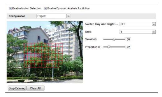
Figure 6-42 Motion Detection Settings-Expert
